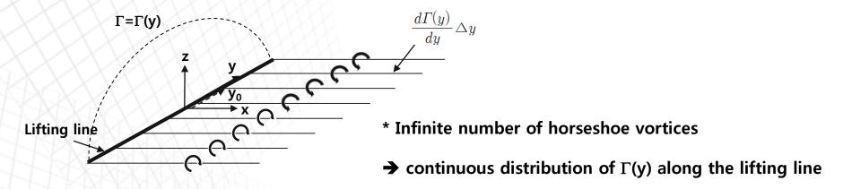
\* The velocity dw at y<sub>0</sub> induced by the entire semi-infinite trailing vortex located at y
