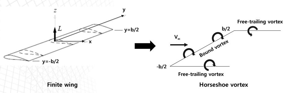
\* The velocity at any point y along the bound vortex induced by the trailing semi-infinte vortices
