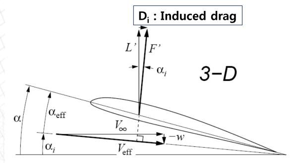
\* Total drag = profile drag + induced drag = pressure drag + skin friction drag + induced drag D<sub>total</sub> = D<sub>p</sub> + D<sub>f</sub> + D<sub>i</sub>
