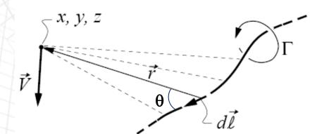
$\vec{dV} = \frac{\Gamma}{4\pi} \frac{\vec{dl} \times \vec{r}}{|r|^3}$  $\vec{V} = \int_{-\infty}^{\infty} \frac{\Gamma}{4\pi} \frac{\vec{dl} \times \vec{r}}{|r|^3}$  $V = |\vec{V}| = \frac{\Gamma}{4\pi} \int_{-\infty}^{\infty} \frac{\sin\theta}{r^2} dl$
