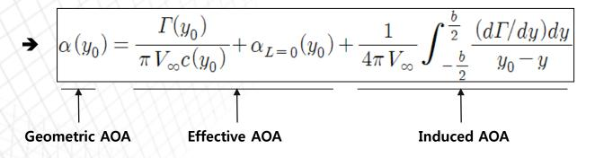
→ The fundamental equation of Prandtl's lifting line theory
